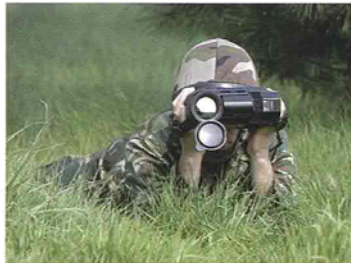
Manufacturers are trying to trim weight from infrared viewers, such as this man-portable unit from Sofradir.
