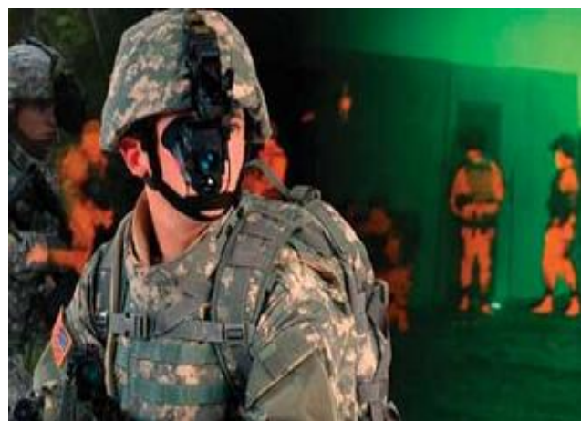
An Enhanced Night Vision Goggle (ENVG) system and optically fused imagery at the background show the green image from an intensifier combined with the amber infrared image. (Courtesy PEO Soldier Portfolio; www.peosoldier.army.mil )
